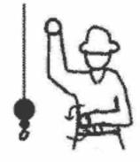
CRAWLER CRANE TRAVEL, ONE TRACK - Indicate track to be locked by raising fist on that side. Rotate other fist in front of body in direction that other track is to travel.
