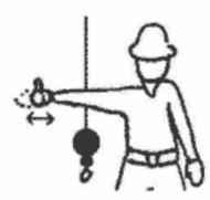
RAISE THE BOOM AND LOWER THE LOAD – With arm extended horizontally to the side and thumb pointing up, fingers open and close while load movement is desired.
