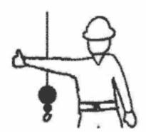
RAISE BOOM – With arm extended horizontally to the side, thumb points up with other fingers closed.
