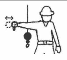
LOWER THE BOOM AND RAISE THE LOAD - With arm extended horizontally to the side and thumb pointing down, fingers open and close while load movement is desired.
