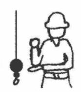
USE AUXILIARY HOIST (whipline) – With arm bent at elbow and forearm vertical, elbow is tapped with other hand. Then regular signal is used to indicate desired action.
