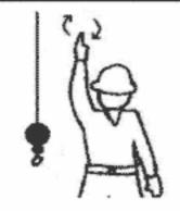
HOIST – With upper arm extended to the side, forearm and index finger pointing straight up, hand and finger make small circles.
