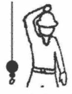
USE MAIN HOIST - A hand taps on top of the head. Then regular signal is given to indicate desired action.
