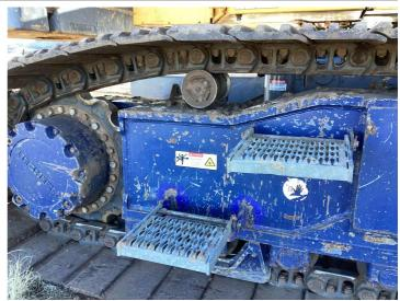
Q16: Are the Track Frame Centering Plates "Pucks" properly located, securely attached and all accompanying hardware tight and without signs of compromise or movement?
