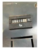
Track Hour Meter Reading
