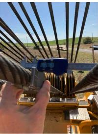
Q8: Has the Boom Hoist Wire Rope been measured on the 2nd layer with the SA Frame unloaded and forward at approximately 135° to check the flattening of the Wire Rope caused by a Long Main Boom configuration without the use of a Derrick? N/A
