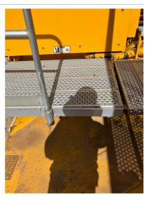
Q3: Do the Anti-Skid Surfaces on the machine still have
