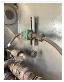
Q23: Are the Carbody and Track Frame Hydraulic and Electrical Caps, Plugs, and Covers present and free of damage?
