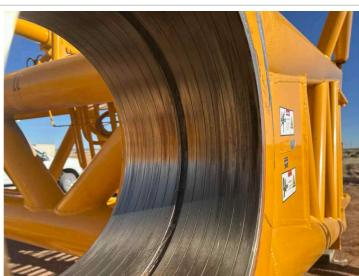
Q9: Are the Boom Stop Cylinders (S Relapse Cylinders) free of deformation, cracks, significantly corroded members, loose fasteners, cracked welds, hydraulic leaks, and significant wear?
