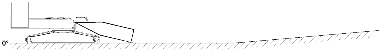
Fig.121635: Disassembling and removing the boom - intermediate sections to the boom - pivot section
