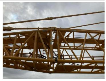
Q11: Are the Derrick Boom Stop Cylinders (D Relapse Cylinders) free of deformation, cracks, significantly corroded members, loose fasteners, cracked welds, hydraulic leaks, and significant wear?
