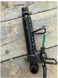
Q18: Are the Mechanical Auxiliary Supports (Frog Legs) in a safe operating condition, free of cracks, complete with screw handle, outrigger pads, and fasteners that are free of apparent damage that could cause failure while in use? N/A
