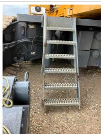
Q53: Are the Steps, Ladders, Handrails, and Guards used to access the Cab and Upper Works present and in a safe and usable condition?
