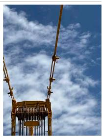
Q2: Are the Boom Stops (Relapse Cylinders) free of deformation, cracks, significantly corroded members, loose fasteners, cracked welds, and significant wear?
