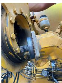
Q24: Are the Hydraulic Motors free of unusual noise, excessive overheating, loose bolts, shaft seals and pump section leaks?
