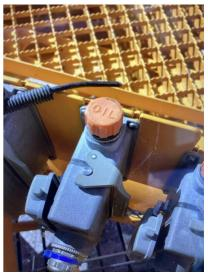
Q11: Does the Electrical / Hydraulic Swivel appear free of leaks, damage, deterioration, corrosion, and dirt and moisture accumulation that would affect its proper operation?
