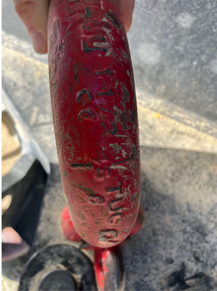
Picture 8 – Picture Documenting Crosby® 17-Ton Screw Pin Shackle Used in the Load Test
