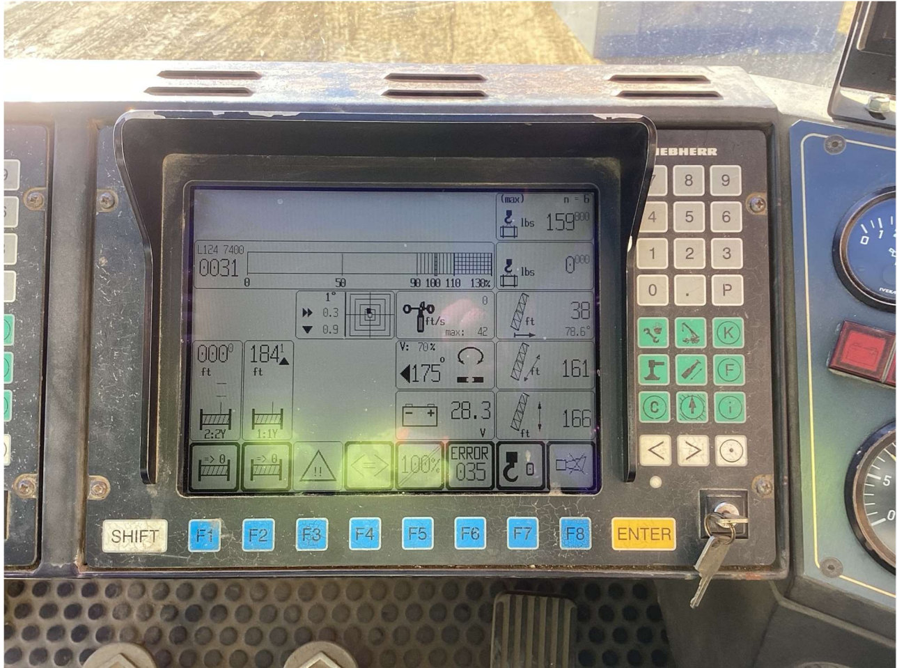
Picture 2 – LICCON Screen Showing No-Load Condition Pre-Test
