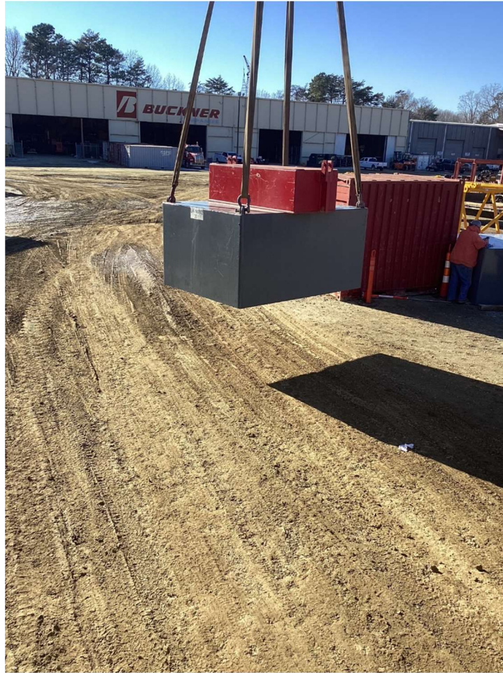
Picture 3 – Picture Showing Counterweight Free of the Ground – Full Load Applied to Lifting Rings
