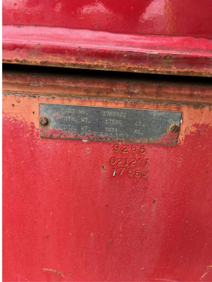
Picture 12 – Picture Documenting Manitowoc 7.974t (17,580 lb.) Counterweight Used as the Additional Ballast in the Load Test
