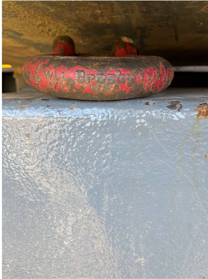
Picture 11 – Picture Documenting Crosby® 17-Ton Screw Pin Shackle Used in the Load Test
