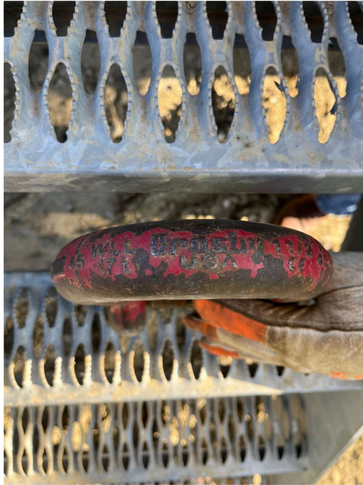
Picture 9 – Picture Documenting Crosby® 17-Ton Screw Pin Shackle Used in the Load Test
