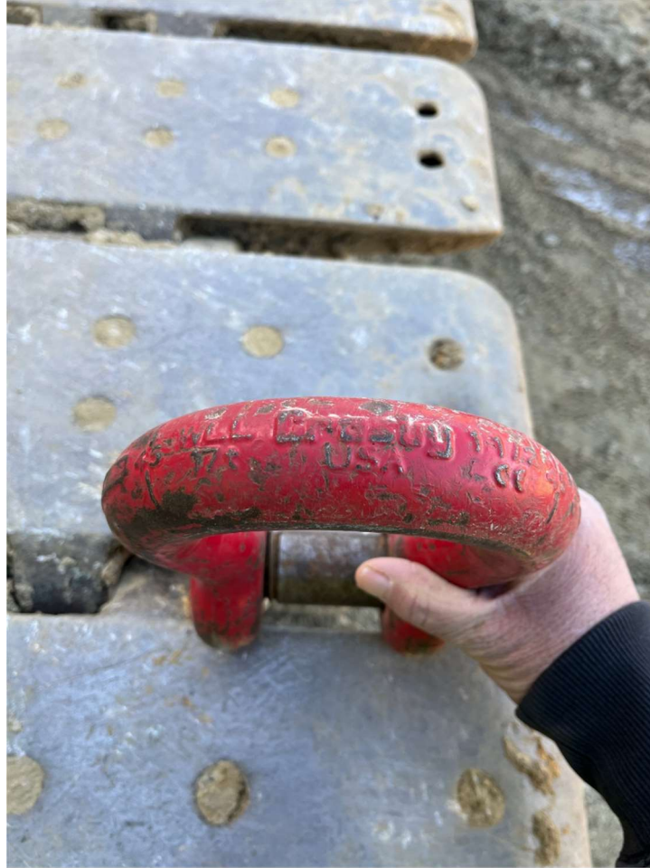
Picture 10 – Picture Documenting Crosby® 17-Ton Screw Pin Shackle Used in the Load Test
