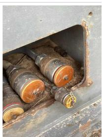
Q24: Are the Hydraulic Motors free of unusual noise, YES excessive overheating, loose bolts, shaft seals and pump section leaks?
