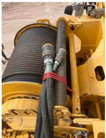
Q24: Is the Aux Winch hydraulic motor, lines, hoses, N/A valves, and connections free of leakage, damage, or chaffing?
