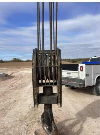
Q7: Are the Cheek Weights free of deformation, cracks, significantly corroded members, loose fasteners, and cracked welds?
