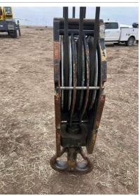
Q7: Are the Cheek Weights free of deformation, cracks, significantly corroded members, loose fasteners, and cracked welds?
