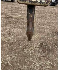
Q10: Is the Hook Throat Opening free of any distortion YES causing an increase of 5% Hook Opening or ¼" Maximum from the manufacturer?
