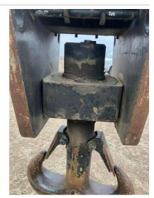
Q13: Is the Swivel Bearing free from cracks and excessive YES wear?
