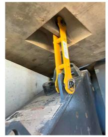
Q56: Are all the Counterweight Trays and Mounting YES Hardware present and installed correctly per manufacturer? Q57: Are all the originally supplied and required YES Counterweight Warning Signs present in a good and legible condition?
