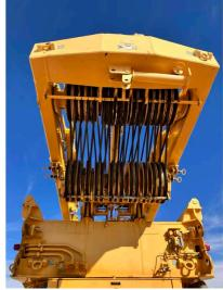
Q4: Are the Outer Bail, Equalizer, Bridle, Lower Sheave N/A Pack, and Shafts free of deformation, cracks, loose components, and loose fasteners?
