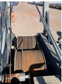
Q7: Has the Wire Rope Diameter been measured in the area where the wire rope is likely to be used during the shift?
