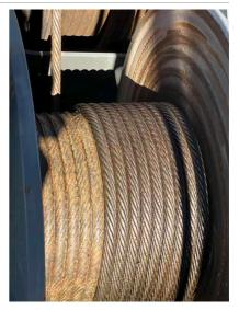
Q7: Has the Wire Rope Diameter been measured in the area where the wire rope is likely to be used during the shift?
