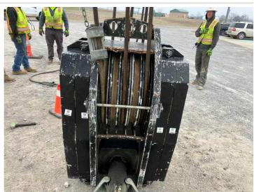
Q7: Are the Cheek Weights free of deformation, cracks, significantly corroded members, loose fasteners, and cracked welds?
