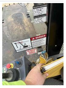
Q23: Is the Electrocution Warning Sign (Inside) posted in the cab and in view of the Operator?
