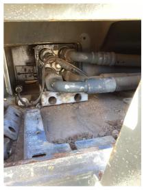
Q22: Are the Track Frame Electrical Connections clean YES and free of damage?
