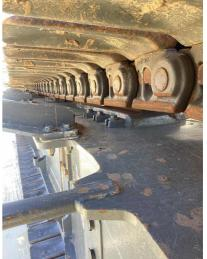
Q12: Are the Track Pads, Pins, and Retainers free of deformation, cracks, significantly corroded members, loose fasteners, cracked welds, and significant wear?
