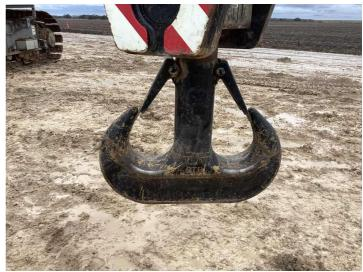
Q9: Is the Hook free of any visibly apparent bend or twist
