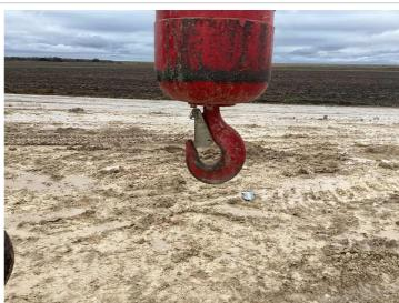
Q4: Is the Hook free of any visibly apparent bend or twist from the plane of the unbent hook (0° Hook Bend or Twist)?
