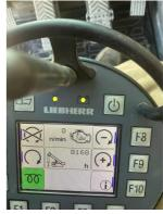
Track Hour Meter Reading
