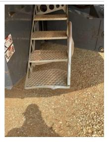
Q3: Do the Anti-Skid Surfaces on the machine still have their slip-resistant properties present and functioning?
