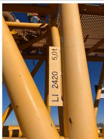
Q5: Are all the Boom Section Warning Labels and Decals present on each section, legible, and installed correctly per manufacturer?
