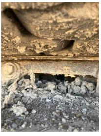
Q12: Are the Track Pads, Pins, and Retainers free of deformation, cracks, significantly corroded members, loose fasteners, cracked welds, and significant wear?
