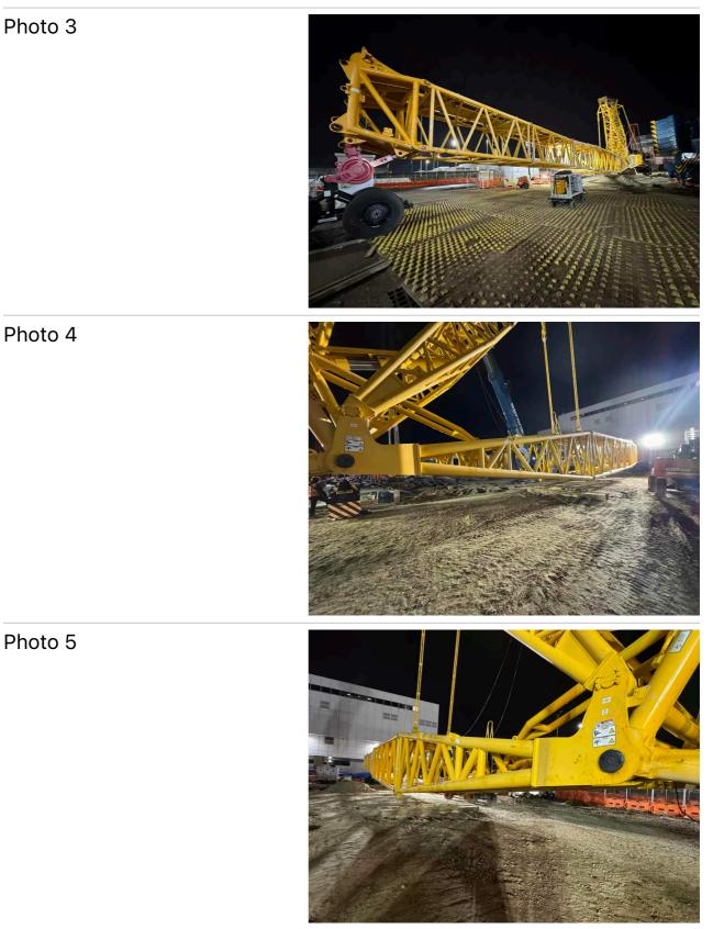
Q2: Are the Chord Members free of deformation, cracks,
