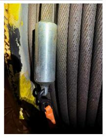
Q5: Is the Main Hoist Wire Rope free of significant distortion of the wire rope structure such as kinking, crushing, unstranding, birdcaging, signs of core failure, steel core protrusion between the outer strands, corrosion, electric arc damage, improperly applied connections, broken wires, or a diameter reduction of 5% from the nominal diameter?
