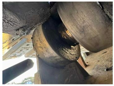
Q11: Are the Drag Bars free of deformation, cracked welds, and significant wear?
