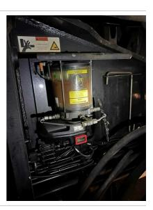
Q20: Have the Lower Roller Grease Line guards been removed, and the Grease Lines checked for leaks, abrasion, significant wear, and dirt/rock buildup?
