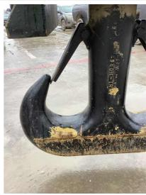
Q11: Is the Hook Wear less than 10% of the original section dimension of the hook or its load pin?
