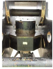
Q13: Is the Swivel Bearing free from cracks and excessive wear?
