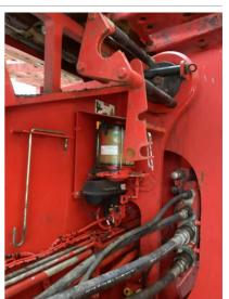
Q20: Have the Lower Roller Grease Line guards been removed, and the Grease Lines checked for leaks, abrasion, significant wear, and dirt/rock buildup?
