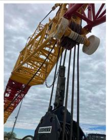
Q2: Are the Chord Members free of deformation, cracks, significantly corroded members, loose fasteners, cracked welds, and significant wear?
