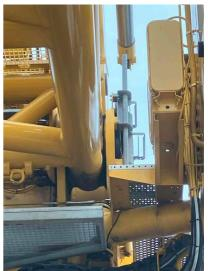
Q9: Are the Boom Stop Cylinders (S Relapse Cylinders) free of deformation, cracks, significantly corroded members, loose fasteners, cracked welds, hydraulic leaks, and significant wear?
