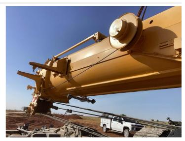
Q7: Are the Telescopic Boom Sections in alignment and free of deformation, cracks, significantly corroded members, loose fasteners, cracked welds, and significant wear?
