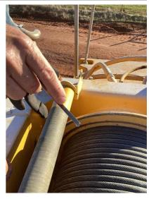
Q16: Are the Main Winch Hydraulic QD Caps / Plugs present and attached to the Hydraulic lines on the Winch, so they don't get damaged or lost?
