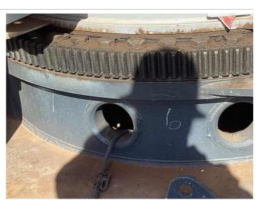
Q3: Is the Slew Ring Connection free of deformation, YES cracks, significantly corroded members, loose fasteners, cracked welds, and significant wear?
