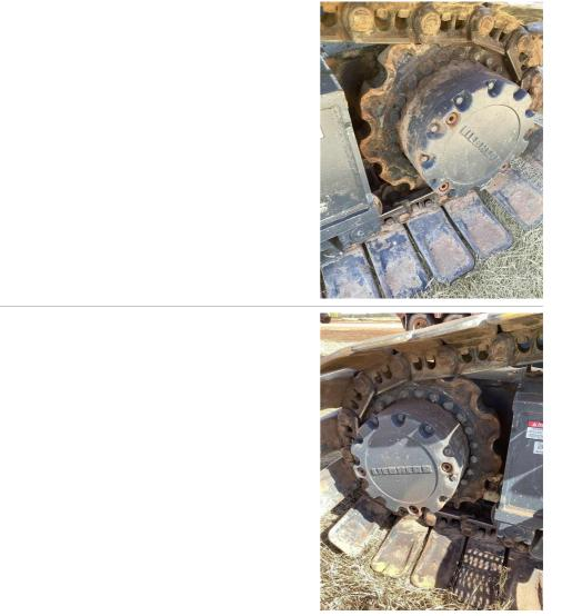
Q9: Are the Drive Tumbler Lugs free of excessive wear?
