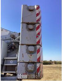
Q56: Are all the Counterweight Trays and Mounting YES Hardware present and installed correctly per manufacturer?
