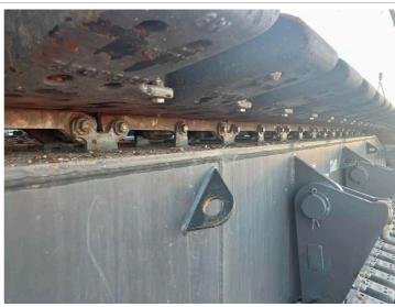
Q12: Are the Track Pads, Pins, and Retainers free of deformation, cracks, significantly corroded members, loose fasteners, cracked welds, and significant wear?
