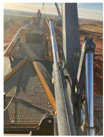
Q10: Are the Boom Foot Pins / D-Pivot Main Pins and Keepers free from cracks and excessive wear?
