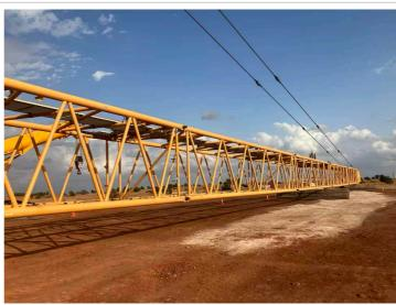
Q2: Are the Lattice Members free of deformation, cracks, significantly corroded members, loose fasteners, cracked welds, and significant wear?
