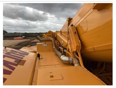
Q8: Are all Hoses free from deterioration and leakage, particularly in hoses that flex during normal operation?
