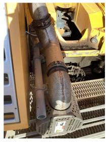
Q8: Are all Hoses free from deterioration and leakage, particularly in hoses that flex during normal operation?
