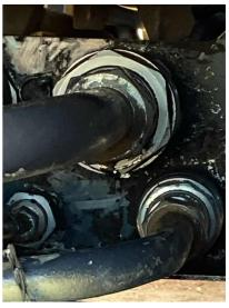
Q22: Are the Track Frame Electrical Connections clean and free of damage?
