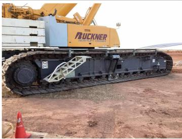
Q16: Are the Travel Locks functioning properly and free of excessive wear?
