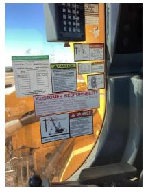
Q23: Is the Electrocution Warning Sign (Inside) posted in the cab and in view of the Operator?
