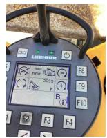
Track Hour Meter Reading
