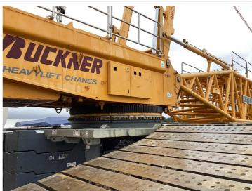
Q3: Is the Slew Ring Connection free of deformation, cracks, significantly corroded members, loose fasteners, cracked welds, and significant wear?
