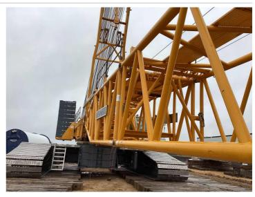
Q2: Are the Lattice Members free of deformation, cracks,
