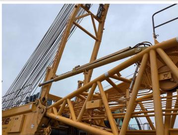
Q10: Are the Boom Foot Pins / D-Pivot Main Pins and Keepers free from cracks and excessive wear?
