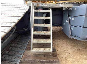
Q53: Are the Steps, Ladders, Handrails, and Guards used to access the Cab and Upper Works present and in a safe and usable condition?
