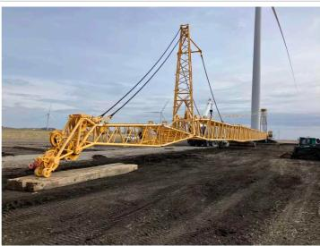
Q2: Are the Chord Members free of deformation, cracks, YES significantly corroded members, loose fasteners, cracked welds, and significant wear?
