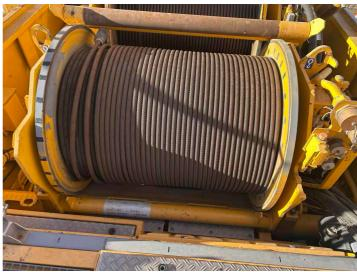
Q24: Is the Aux Winch hydraulic motor, lines, hoses, valves, and connections free of leakage, damage, or chaffing?
