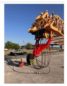
Q13: Is the Auxiliary Boom Head / Extended Upper Boom Point (EUBP) free of deformation, cracks, significantly corroded members, loose fasteners, cracked welds, and significant wear?
