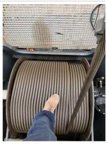
Q30: Does the Auxiliary Hoist have a Minimum of Two (2) Rope Wraps left on the drum when the load and/or boom is in its lowest position? N/A
