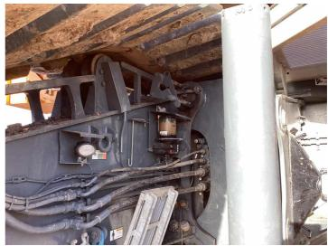
Q20: Have the Lower Roller Grease Line guards been removed, and the Grease Lines checked for leaks, abrasion, significant wear, and dirt/rock buildup?
