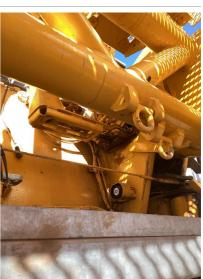
Q11: Are the Derrick Boom Stop Cylinders (D Relapse Cylinders) free of deformation, cracks, significantly corroded members, loose fasteners, cracked welds, hydraulic leaks, and significant wear?
