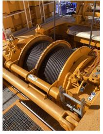
Q44: Is the Boom Hoist Reeving according to manufacturer specifications and without kinking, crushing, unstranding, birdcaging, signs of core failure, and steel core protrusion between the outer strands?
