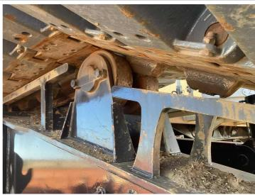
Q11: Are the Drag Bars free of deformation, cracked welds, and significant wear?
