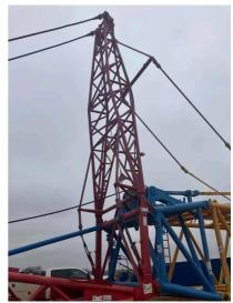
Q5: Are the Jib Stops free of deformation, cracks, significantly corroded members, loose fasteners, cracked welds, and significant wear?
