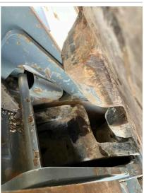
Q9: Are the Drive Tumbler Lugs free of excessive wear?
