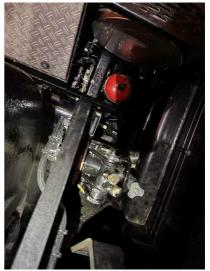
Q24: Is the Aux Winch hydraulic motor, lines, hoses, valves, and connections free of leakage, damage, or chaffing?
