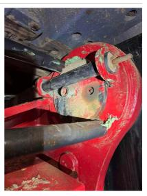
Q6: Are the Track Frame Lifting Lugs (Dog Bone) free of
