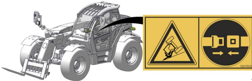
Safety belt sign
