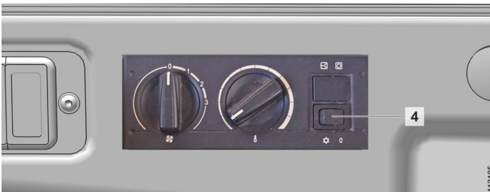
Main switch for the air conditioning system
