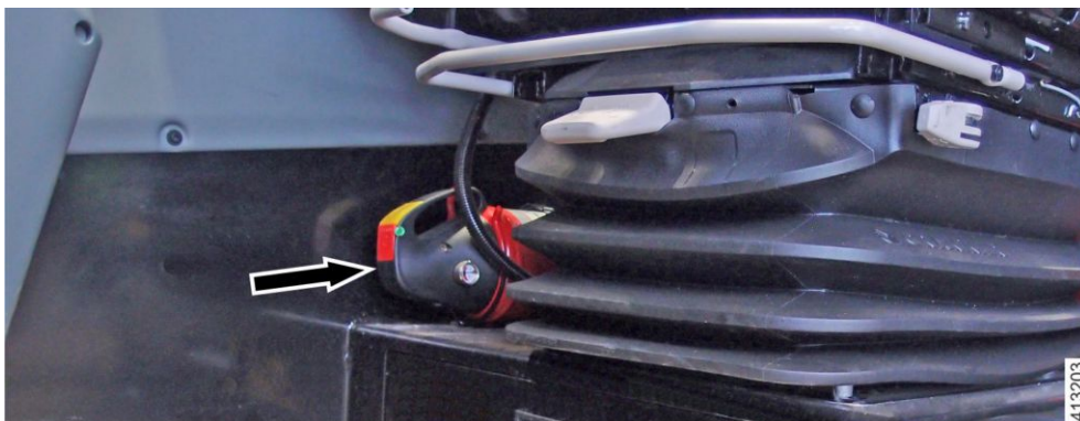
Mounting location of fire extinguisher
