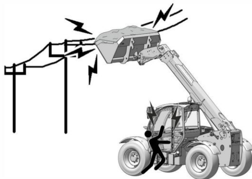
Working in vicinity of overhead power lines
