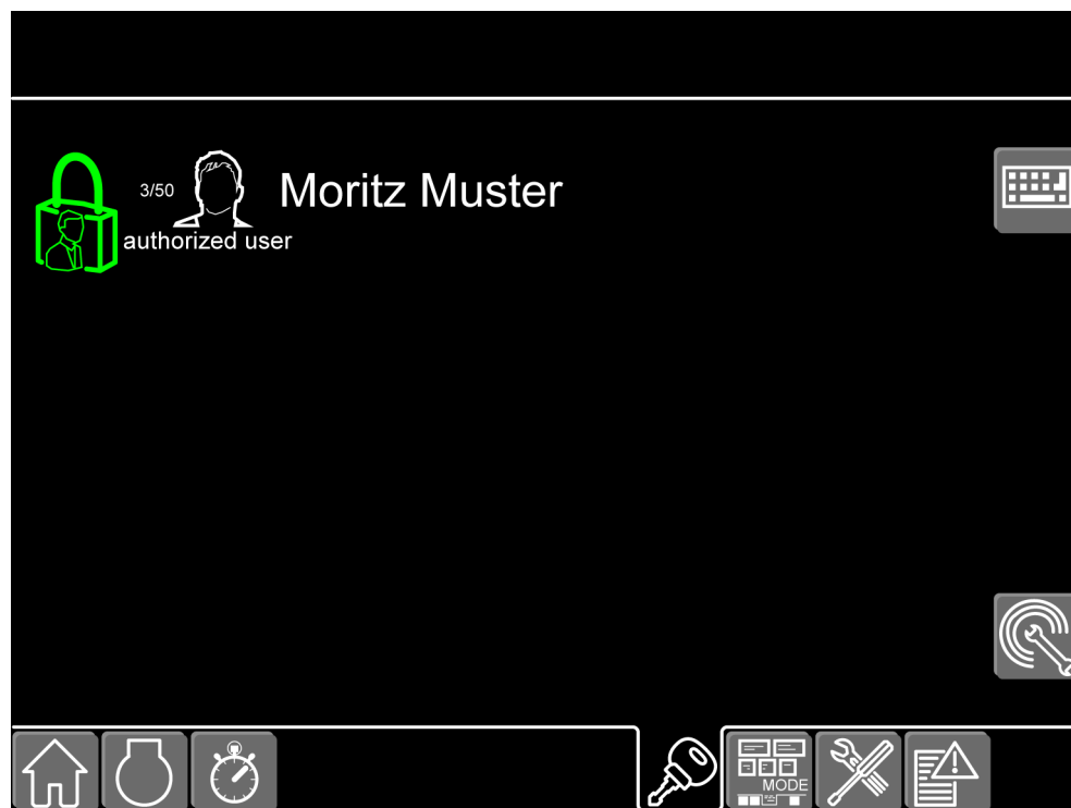
Fig. 1900: Access control screen - with retrofit kit access control (access with blue, user-specific ignition key)
