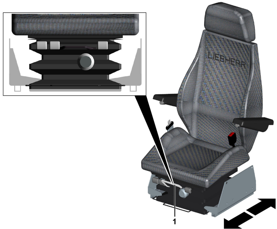
Fig. 2243: Adjusting the operator's seat horizontally
