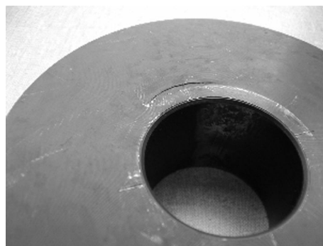
Fig. 6032: Crack on a bush
