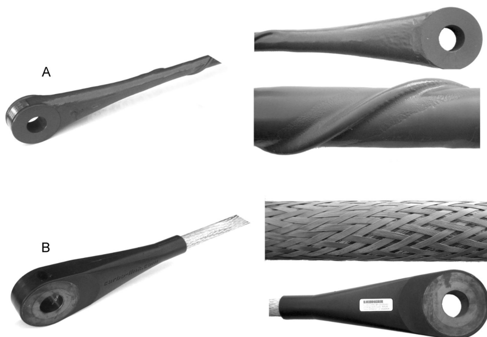
Fig. 5938: Generation A and generation B of the CF pedant straps
