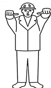
Fig.144250: Retracting the boom
