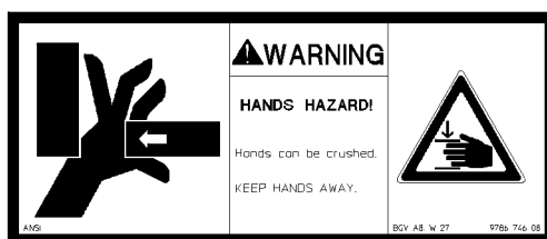
Fig.106030: Crushing danger for hands
