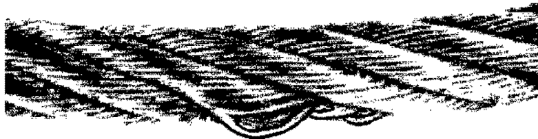
Fig.120991: Distorted or protruding strand
