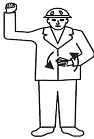
Fig.144248: Moving one crawler chain
