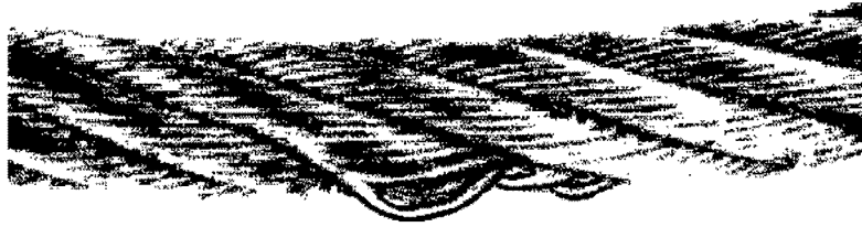
Fig.120991: Distorted or protruding strand
