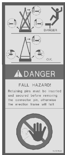
Fig.158615: Connector pins for erection rack / guy rods
