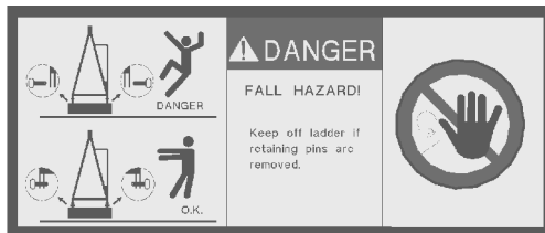
Fig.158614: Retaining pins for erection rack
