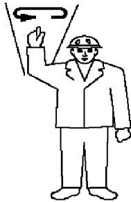
Fig.111706: Lifting / lowering a load with even speed
