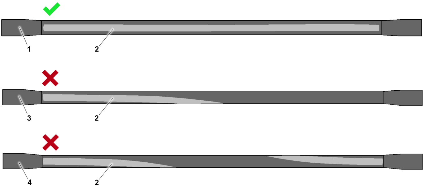
Fig.160904: Twisting marking for a straight fiber guy rope, example of a twisted fiber guy rope!
