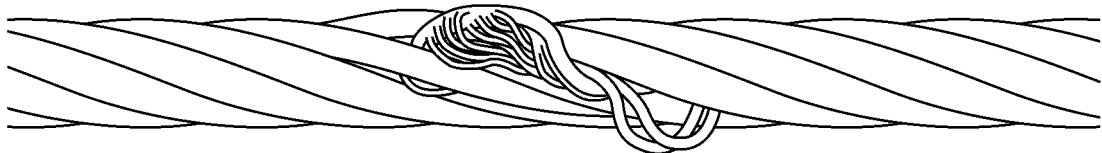
Fig.120990: Protrusion of an insert (rope single layer)
