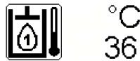
Fig.148386: Hydraulic oil temperature, hydraulic circuit 1 icon, display value and unit of measure
