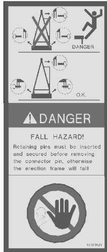
Fig.158615: Connector pins for erection rack / guy rods
