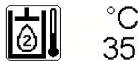
Fig.148387: Hydraulic oil temperature, hydraulic circuit 2 icon, display value and unit of measure
