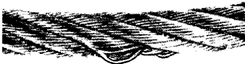
Fig.120991: Distorted or protruding strand
