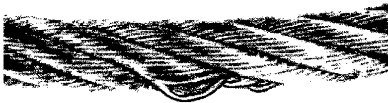
Fig.120991: Distorted or protruding strand
