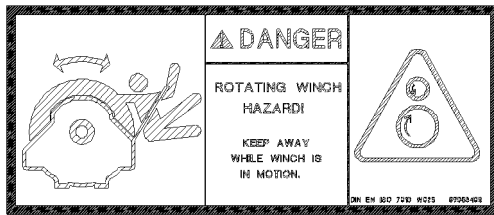
Fig.144738: Entanglement hazard during winch operation
