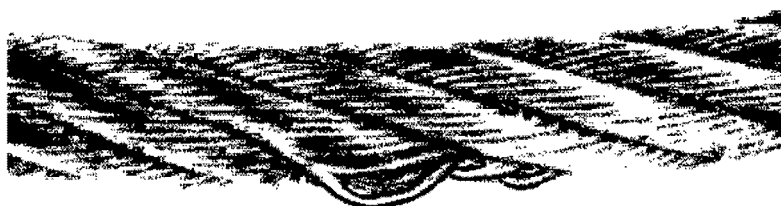
Fig.120991: Distorted or protruding strand
