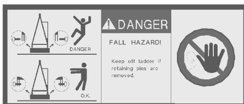
Fig.158614: Retaining pins for erection rack
