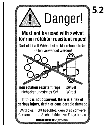
Fig.154084: Symbols for non-twisting ropes with rope end connections
